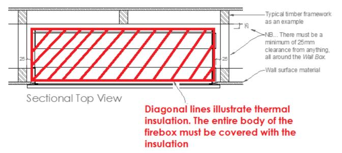
Note: The drawing on pg. 8 is an example of a typical installation using a timber framework and covering the firebox body with insulation. All installations must comply with the relevant building regulations and restrictions of the country where the installation is to take place!
