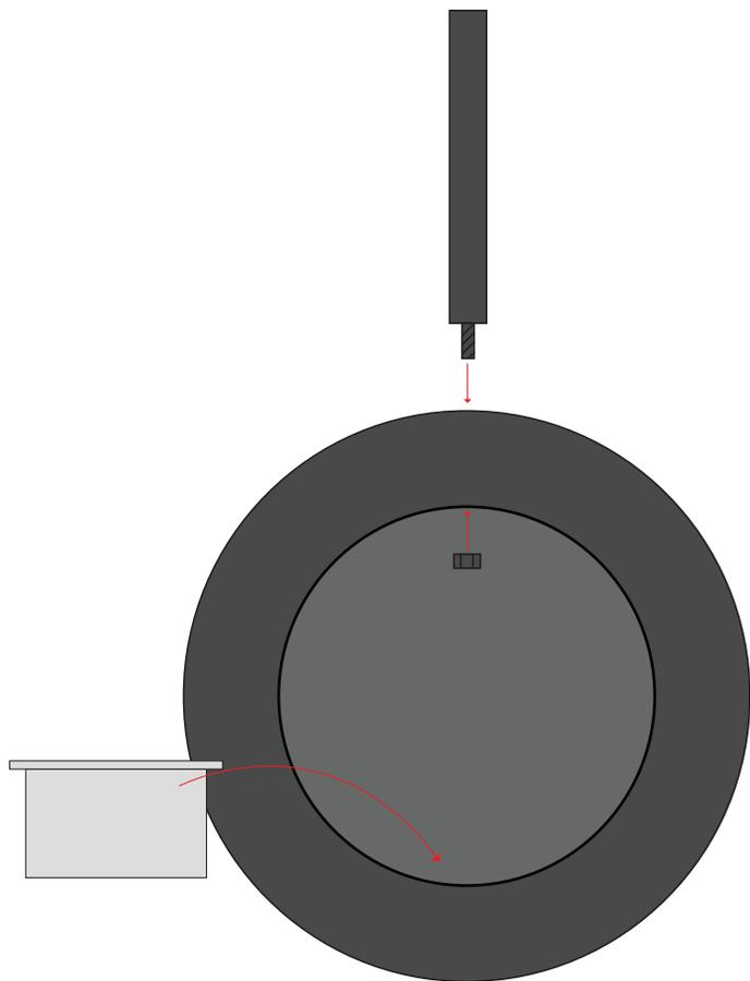
Attach the ceiling rod to the fireplace using the included nut.
